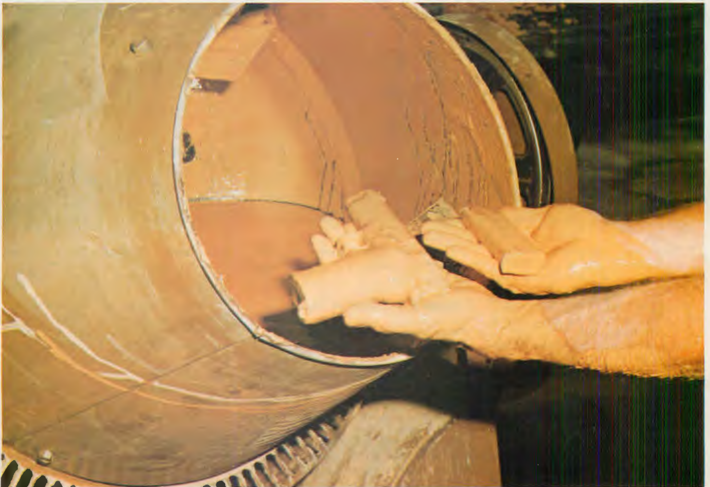
ABOVE: Test pistols must function in cold room's minus 60 degrees F. This hurdle alone eliminated some contenders. BELOW: Test pistols undergo mud bath in cement mixer. Afterwards they must shoot (minor manual assistance is allowed).
